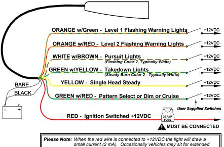
ase Note: When the red wire is connected to +12VDC the light will draw a small current (2 mA). Occasionally vehicles may sit for extended periods of time (i.e. more than a few days), thus we recommend that the red wire be routed through an ignition switched power source.
